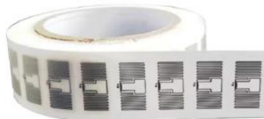
U2715 UHF Inlays Tags Stickers Chip: U8,U9 Antenna size: 24x12mm Label size: 27x15mm Reading distance: 3m
