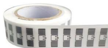
U3314 UHF Inlays Tags Stickers Chip: U8,U9 Label size: 33x14mm Reading distance: 3.5m
