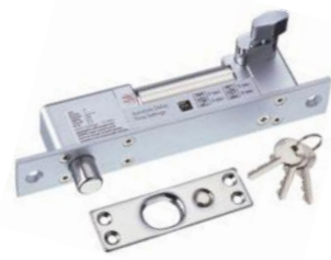
BL-2500A / 2500B Dead Bolt Lock (power on to open) BL-2500A: (power to open) N.C. door position output point BL-2500B: (power to open) Door position detection and bolt position(N.C. & N.O.) output points
