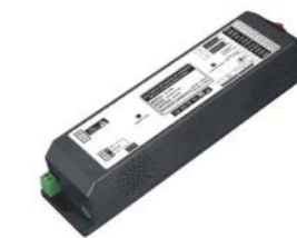
M-236E Automatic door back-up power with lithium battery 1. Input Voltage: AC220V 50Hz 2. Output Voltage: DC24V 2.6AH; DC12V 5.2AH 3. Working Mode: Automatic working or keep opening 4. Dimension: 243x59x45mm
