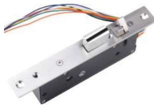
BL-2400 Positioning Smart Electric Mortise Lock 1. Lock body size:200x28x50.5mm 2. Lock tongue size:protruding length 21mm, width 30mm 3. Embedded size:145x26.5x48mm
