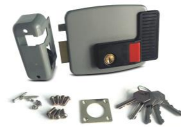
ER-D3 Electric RIM lock with Nickle plating 1. Double-separated brass cylinder 2. Working voltage: 12V DC 3. Door thicknesses: 35 to 50mm
