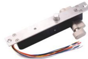
BL-2900 LED Indicator Electric Mortise Lock 1. Working current: start 1.2A holding 0.2A 2. Working Voltage: DC12V/24V 3. Delay function: 0/3/6/9 delay can be selected
