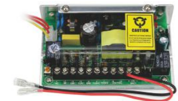
208K NEW Switching Power Supply 1. Input: AC110V-240V / 50Hz-60Hz 2. Output: DC12V / 5A 3. Dimension: 132 x 74 x 39mm 3. Weight: 0.4kg
