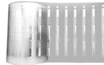
E44(Dry Label) UHF Inlays Tags Stickers Chip: M4E Antenna size: 6x105mm Label size: 9x108mm Reading distance: 8m
