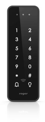
PRT84ME is an identification terminal which enables access system users to be recognized by means of PIN codes and EM 125 kHz or 13.56 MHz MIFARE® CSN/SSN proximity cards. The reader is equipped with a touch numeric keypad, two input lines and two function keys marked with the symbols Bell and Light. The function keys can be used for purposes other than those indicated by their associated symbols.
