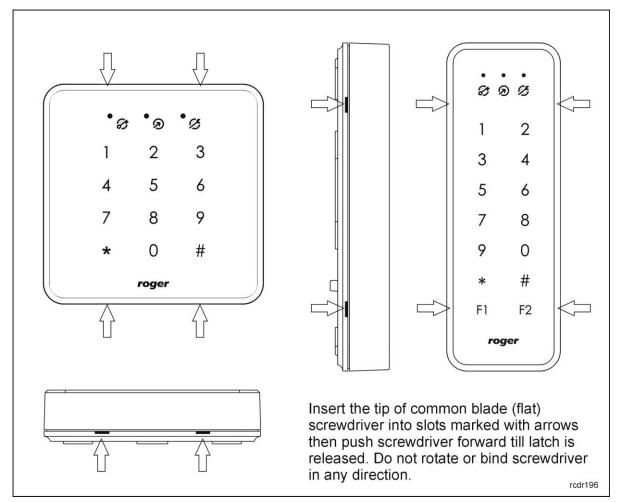
Fig. 6 PRT82MF/PRT84MF enclosure disassembly
