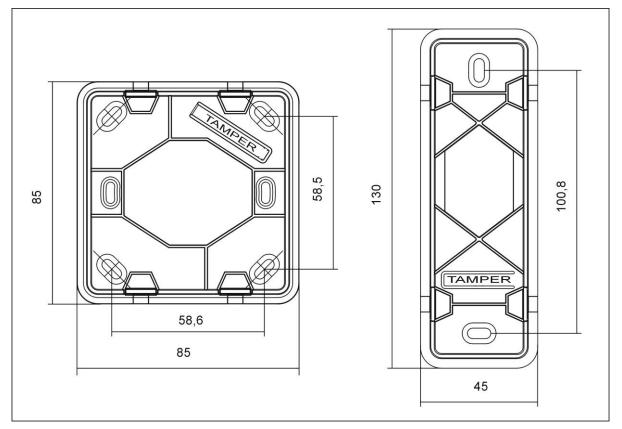
Fig. 9 Dimensions and tamper details
