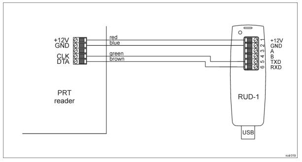
Fig. 3 Connection of reader to RUD-1 interface
