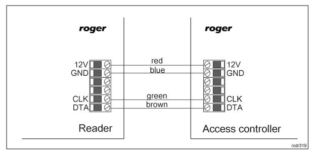
Fig. 1 Connection of reader to access controller (RACS CLK/DTA)
