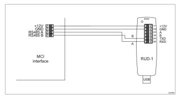
Fig. 2 Connection of the MCI-3 to RUD-1 interface for firmware update
