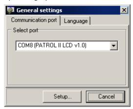
After COM port is properly selected click on *Setup* button and reader will enter online mode (LCD message: **Online mode** and the *Connect icon* in *Patrol Master* program is greyed) and you can continue working with a device. Whenever the connection with the reader is discontinued the *Connect icon* is re-enabled and you can click on it to establish communication link with the device.
