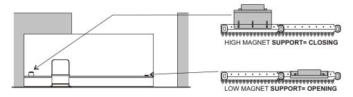
N.B. THE HIGH MAGNET SUPPORT HAS ALWAYS TO BE USED FOR THE CLOSING MOVEMENT
