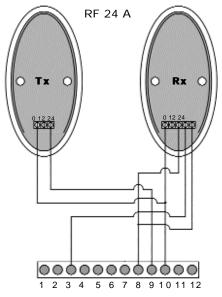
N.B.: Jump terminals 3 and 9 if the photocell in CLOSING has not been installed.
