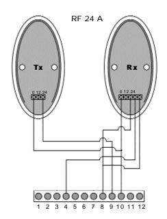
N.B.: Jump terminals 4 and 9 if the photocell in OPENING has not been installed
