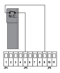
**3.7.2 Mechanical safety edge in OPENING** Wire the safety edge to 6-9, terminal JP5.
