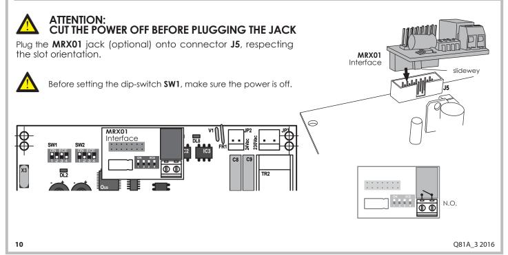
3.10.1 Auxiliary radio channel AUX To use the MRX01 interface as second radio channel, proceed this way:
