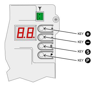
If you wish to reduce or increase the value of the setting use lacktriangle **A ttention!** when you reach the desired setting, wait shortly while the screen displayes the current value and setting alternatively. If you wish to move to a different setting, press and then as previously outlined.
