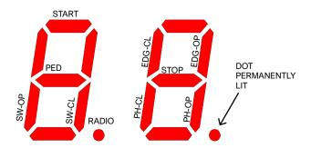
The symbol on the left outlines commands and limit switches (SW-OP and SW-CL stand for opening and closing limit switch). If the input is active the symbol is lit.
