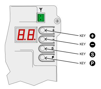
If you wish to reduce or increase the value of the setting use lacktriangle **A ttention!** when you reach the desired setting, wait shortly while the screen displayes the current value and setting alternatively. If you wish to move to a different setting, press lacktriangle and then lacktriangle as previously outlined.
