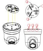
Step 3. Rotate camera clockwise until hear a click sound
