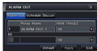
Fig 4-28 system configuration-alarm out
