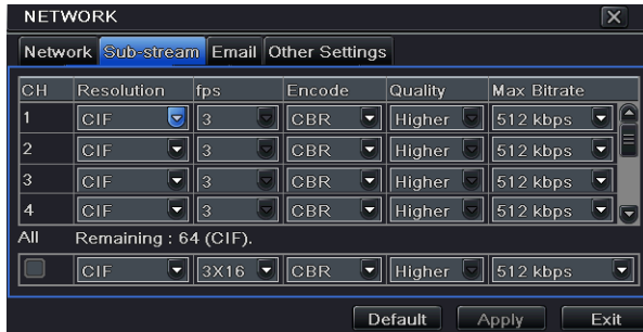
Fig 4-30 network configuration-sub stream
