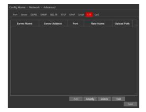
To add a new FTP server click on "Add" and input the FTP server's server name, address, port number, username, password, and upload path, click OK to confirm the setting.
