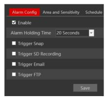
The first tab is the "Alarm Config". Enable or disable the alarm and set the alarm holding time. The holding time means that the alarm signal will stay active and no additional alarms will be generated during that time.
