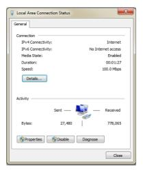
Select "Properties" and then select internet protocol according to the actual situation (most probably you are using IPv4). Next, click "Properties" button and set the network of the PC as shown below.
