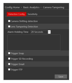
2. Enable the required detection analytics out of Camera Shifting/Lens Tampering/Masking detection.
