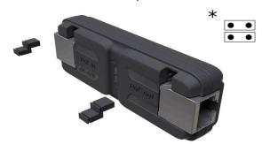
\* When reattaching jumpers, please note horizontal placement as shown below: When all four jumpers are connected GPeR works in both directions.
