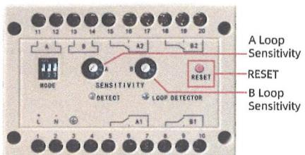
Reset button: When the power is turned on, the auto detector will automatically reset to no car state. After each adjustment of sensitivity or DIP switch, manually press the reset button without car.
