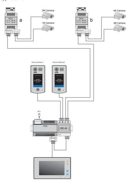
NOTE: The system can connect SC6V(SC6V connected two TYPE B Cameras), but at this time, the DIP6 of DT-SCU must be set to ON.
