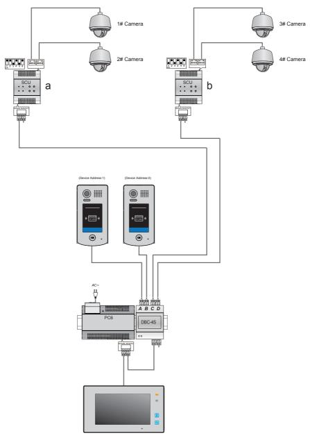
4.3 Multi door station and two SCU(connected two TYPE B Cameras) applications:
