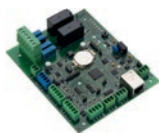
RS485 door controller
