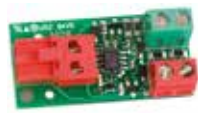
BUS XIB interface (for E045 or E045S or E024S boards with photocell no BUS)
