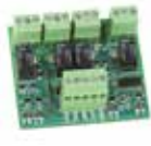
I/O expansion card - 4 OUTPUT 24VDC 1A - 4 INPUT
