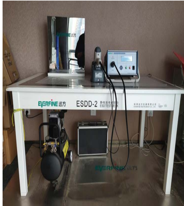
ESD test station
