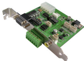
RS-485 converter + TV-OUT board for 32 channel
