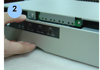
Pull out the HDD tray
