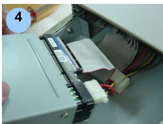
Connect the HDD to the power bus and data bus and secure the connection
