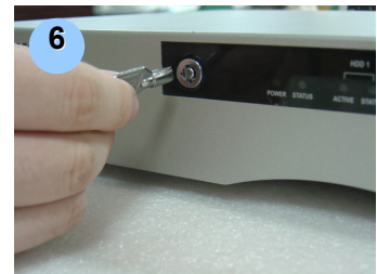
Close and lock the HDD tray
