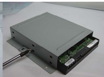
Pull out the HDD tray
