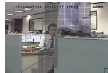
When any movement is detected, you will see the grids are flashing.
