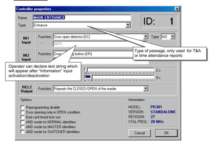
**Reprogramming disabled** – after this option is set reprogarmming of controller is disabled. This option can be removed only by EEPROM RESET.
