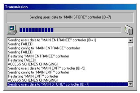
Controllers are equipped with internal memory banks which store configuration settings of controller and users codes. Without communication with system Host (PR Master or CPR-32 control panel) controllers can operate in stand alone mode. In this mode time zones and events recording doesn't function. Before system will start first time every controller must be download with settings. There are few other situation where configuration settings in controller must be updated:
