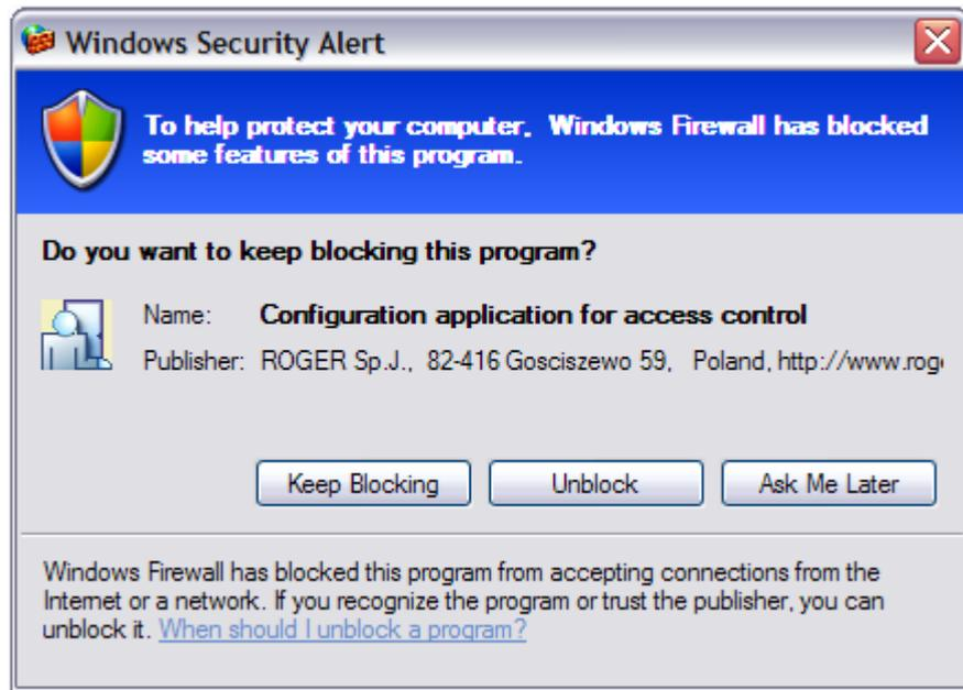
During the PR Master start, program trying to open ports to listen and communicate with Remote Monitor applications.
